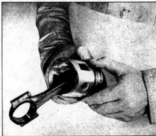
Removing Piston Rings
