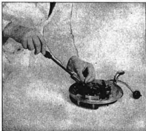
Soldering Leads to Coil
