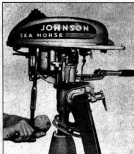
Removing Gas Tank
