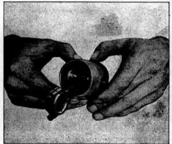
Removing Piston Rings
