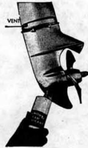
Inserting Gear Lubricant
