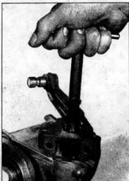
Illustrating Use of Tool No. S-261 for Removing Inner Tube from Drive Shaft Casing
