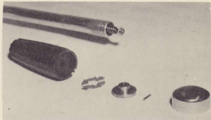
Clutch parts in the twist grip.
