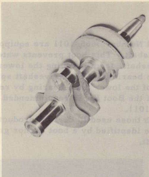
CRANKSHAFT COLLAR INSTALLED
