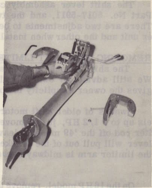
Replacing tilt arm assembly.
