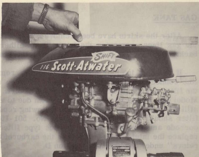
Measuring gas tank height.
