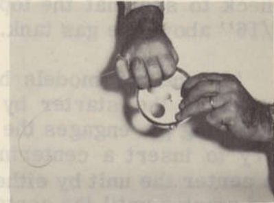
Winding spring in retainer.
