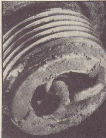
OILY, DIRTY, WORN-OUT SPARK PLUGS
