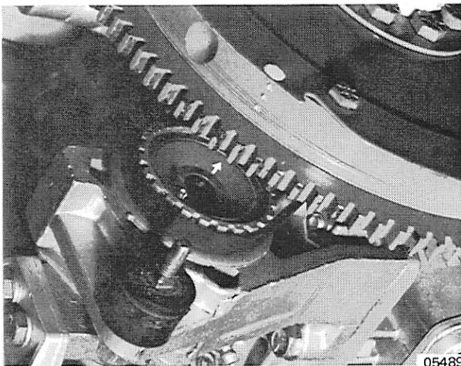
Figure 2. Alignment and Timing Marks on Flywheel and Pulley
