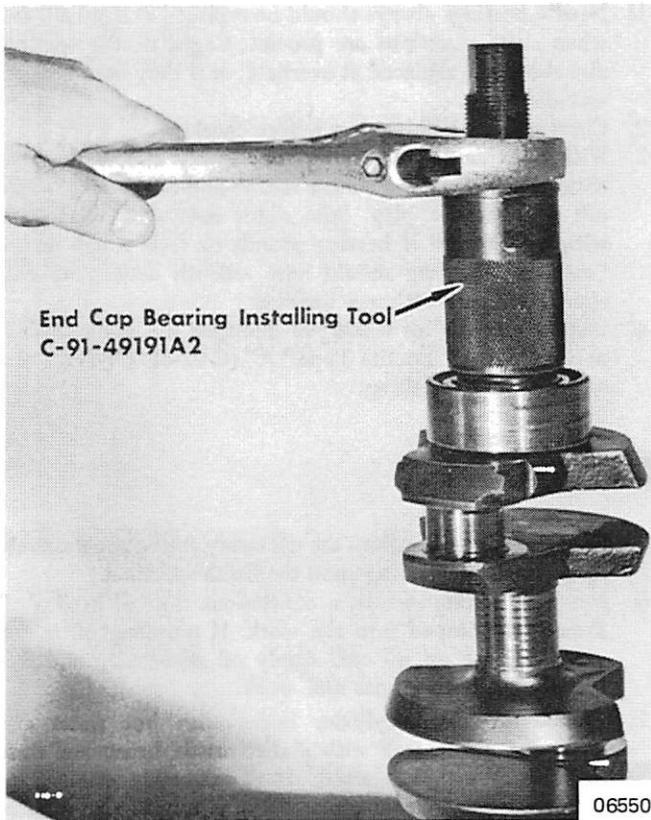
Figure 1. Installing End Cap Ball Bearing
