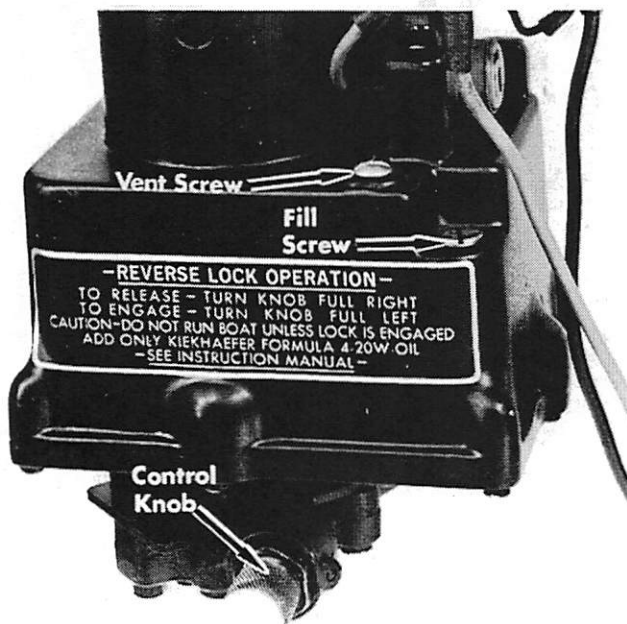
Figure 1. Pump Installed in Vertical Position
