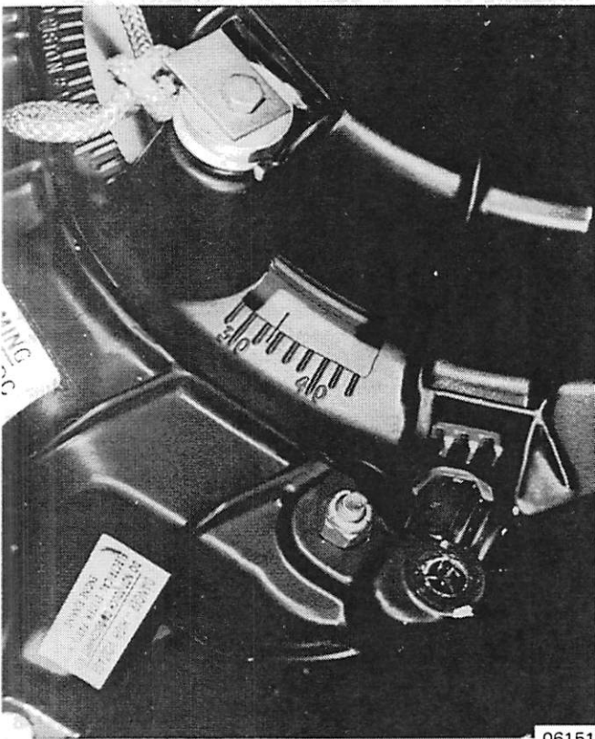
Figure 6. Timing at 33° BTDC
