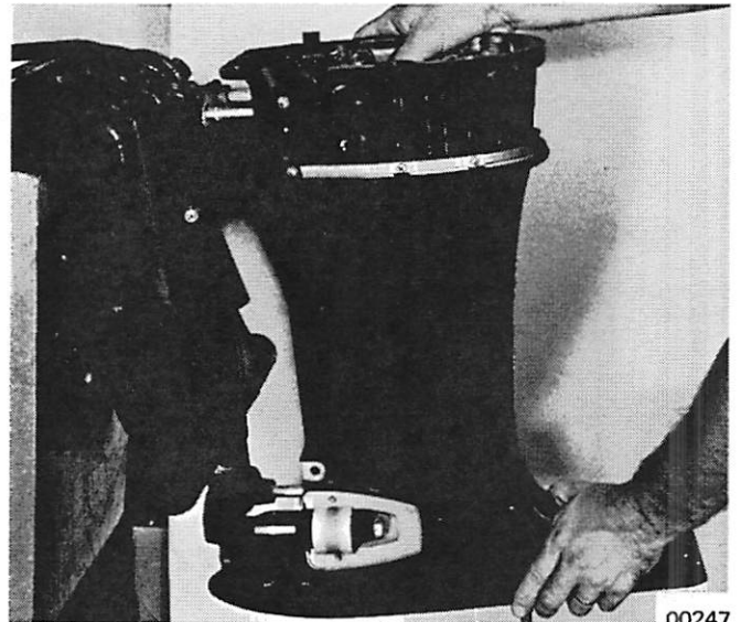
Figure 4. Removing Drive Shaft Housing
