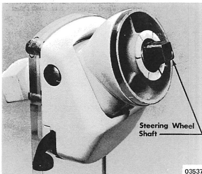
Figure 4. Steering Wheel Shaft Installed
