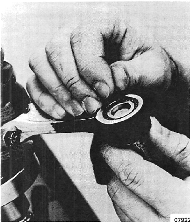
Figure 5. Installing Piston Pin Bearings
