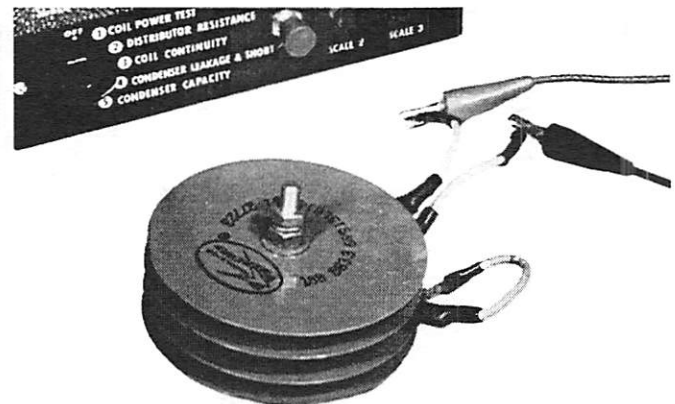
FIGURE 29. Testing Rectifier Selector Switch on No. 3
