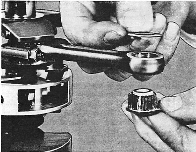
Figure 15. Inserting Piston Pin Bearings & Sleeve into Connecting Rod
