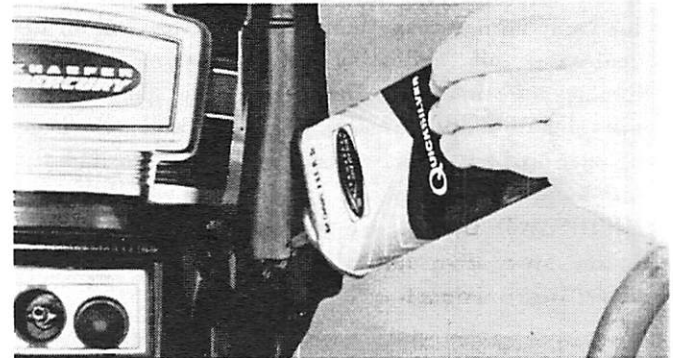
Figure 7. Control Handle Lubrication
