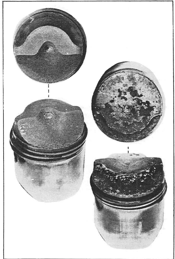
FIGURE 18. Pistons Removed from Motor Using Quicksilver Oil (Left), Regular Grade Oil (Right)
