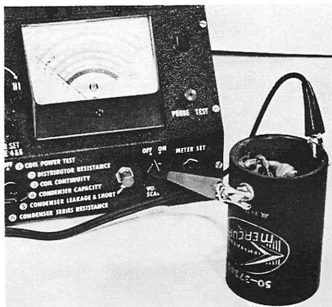
Figure 2. Check for Shorted Field
