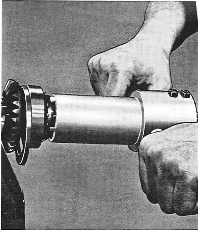
Figure 3A. Removing & Installing Gear Lock Nut
