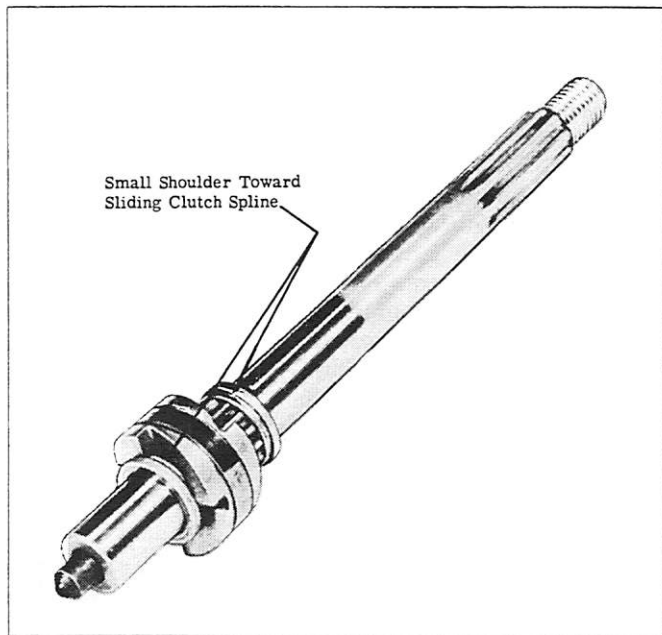
Figure 15. Thrust Washers Correctly Installed on Propeller Shaft
