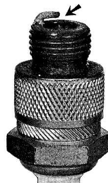
Eroded or burned center electrode to affect spark gap and sparking performance.
