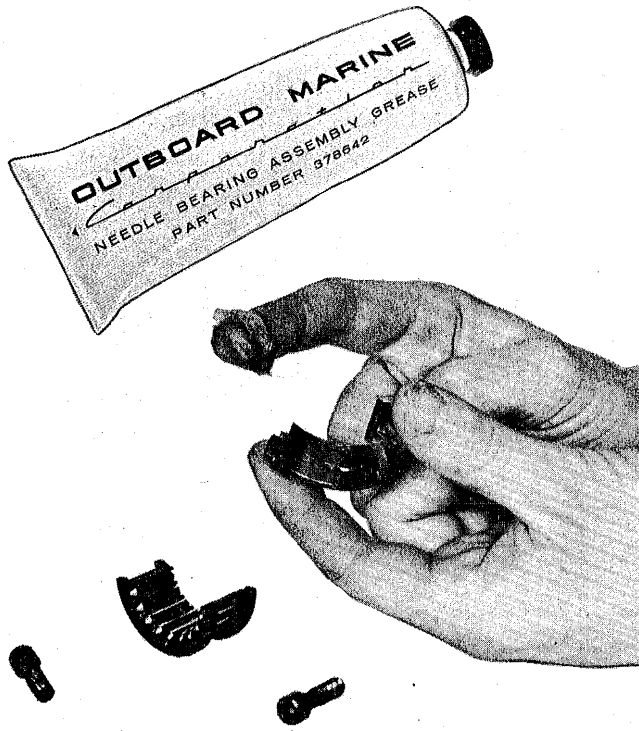
Using Bearing Assembly Grease to Hold Needles in Place During Assembly.
