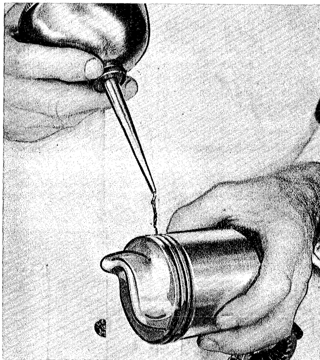
Oiling Piston Ring Grooves—Piston Rings Installed.
