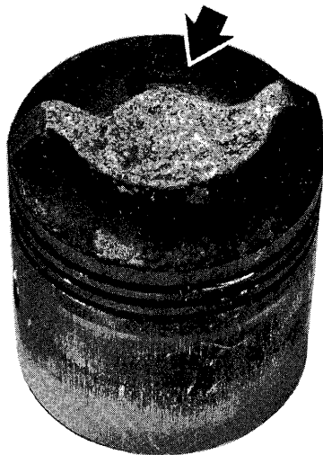
Illustrating the result of extensive pre-ignition. Note piston head erosion.
