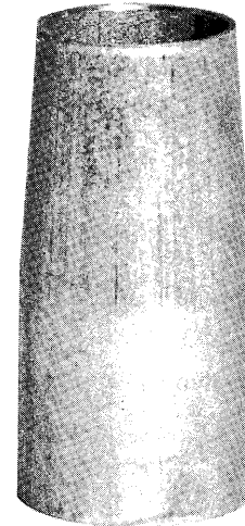
Tool No. 376605 (Sleeve) for assembling Oil Seal on the older crankshafts — provided with "step" at end of Journal.
