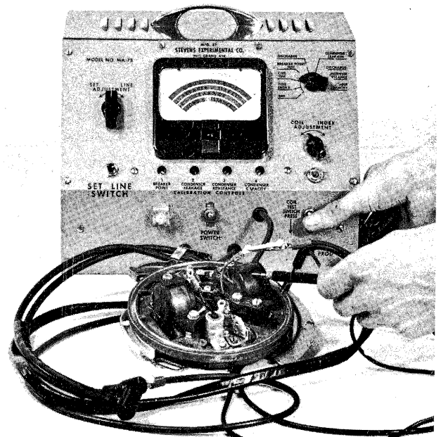
Probing for Surface Leaks.
