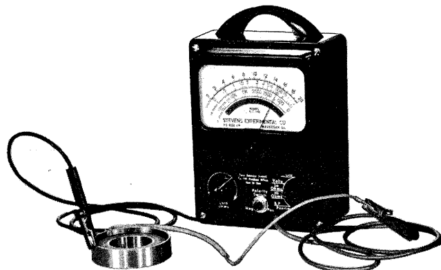
Checking Electromagnet with Stevens VOHM Meter.
