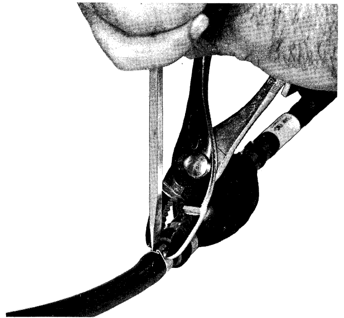
Using screw driver to force end of Clamp into position for securing.
