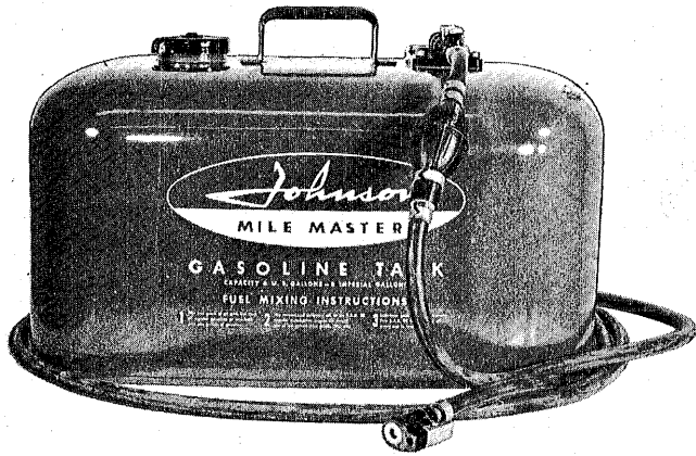
Fuel tank and fuel line assembly - capacity, 6 gallons.
