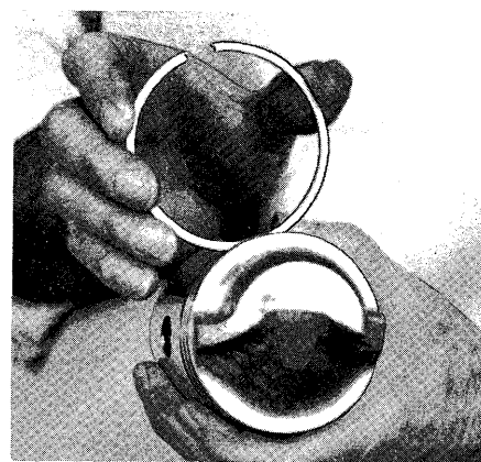
Checking Ring Clearance in Piston Ring Grooves.
