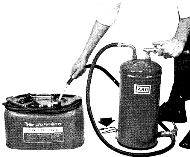
Illustrating Fuel Tank Drainage with Fuel Tank Pump. Note static Ground Wire (arrow) — a safety feature to eliminate static sparking.
