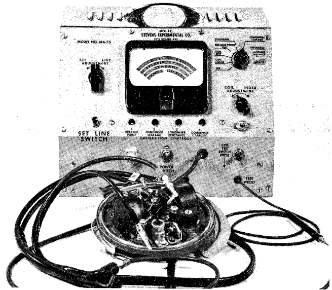
Checking the Condenser.
