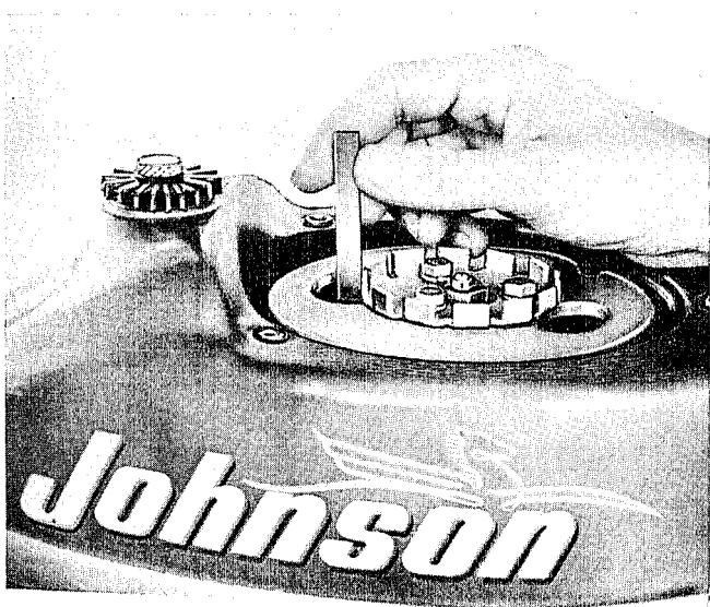
Checking Breaker Point Gap with Feeler Strip— Correct Gap Setting is .020" Full Open.
