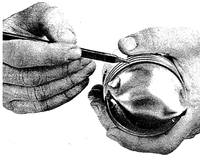
Removing Carbon from Ring Grooves in Piston.
