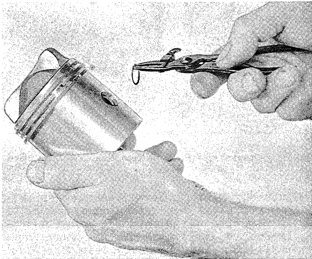
Removing and/or Installing Wrist (Piston) Pin Retainer.
