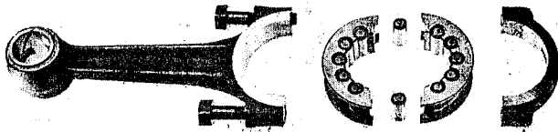
Rollers Placed in Split Cage Ready for Assembly. What Appears to be Free Rollers Actually Find Their Places in Assembly as the Cage or Retainer Sections are Clamped Together on Attaching and Securing of Connecting Rod Cap.
