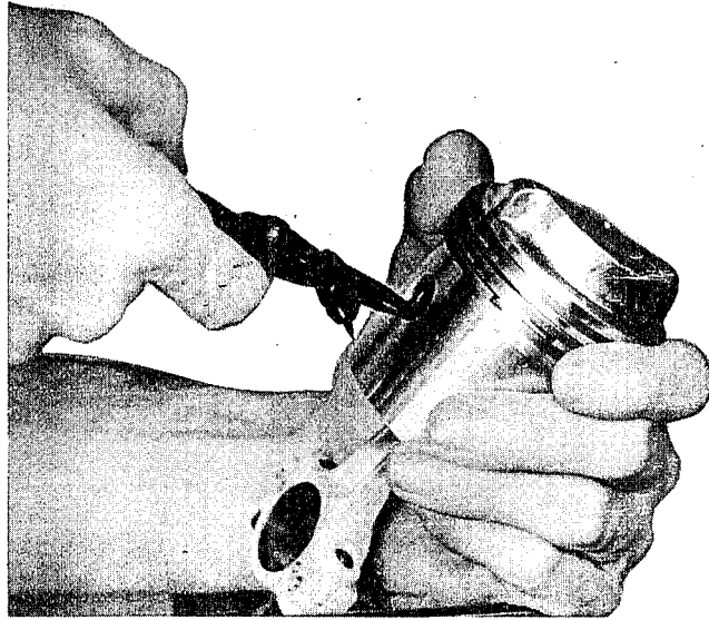
Removing the Wrist Pin Retainer with Tru-Arc Pliers.
