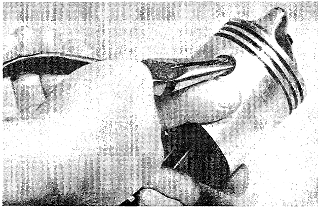
Removing—Installing Wrist Pin Clip (Retainer).
