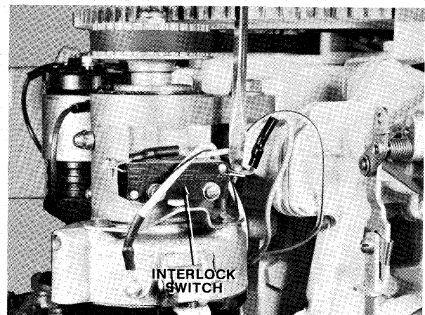
Figure 2—Removing Lead Wire from Interlock Switch
