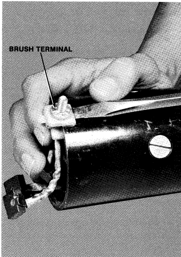
Figure 2—Removing Armature Brush Terminal Assembly
