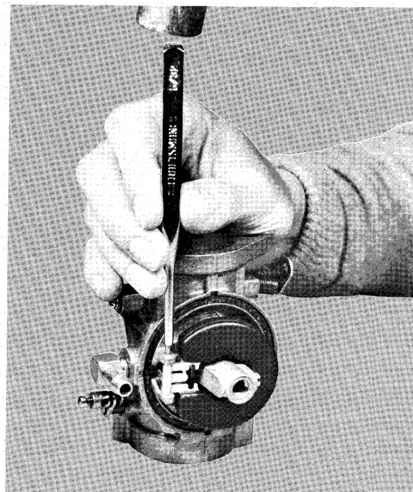
Figure 5—Removing Groove Pin
