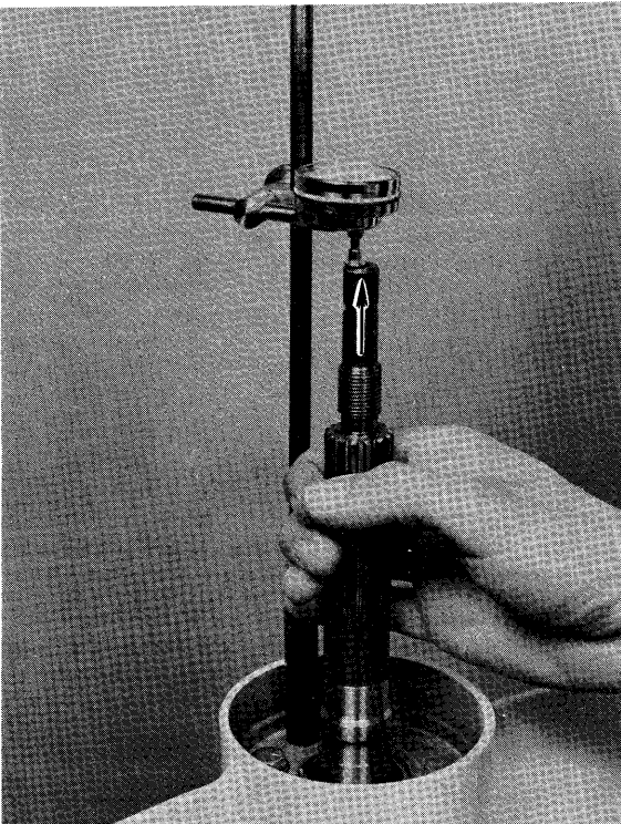
Figure 32—Checking End Float
