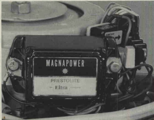
Figure 17. Removing C-D Module from Power Head.
