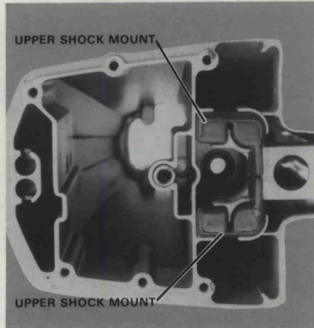
Figure 5. Upper Shock Mounts Installed.
