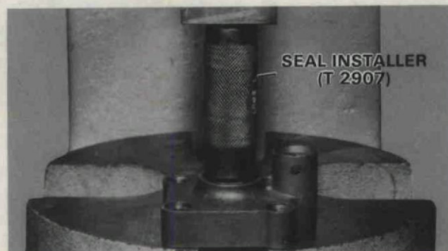
Figure 47. Installing Driveshaft Seal.
