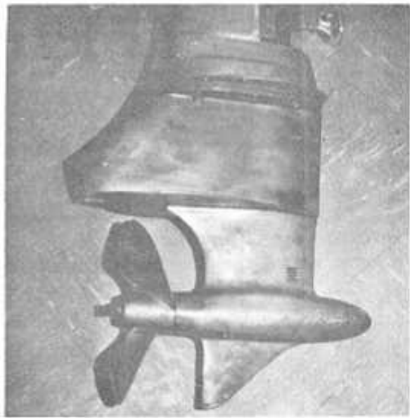
Standard unit with long intermediate housing, rounded nose piece, and regular prop.
