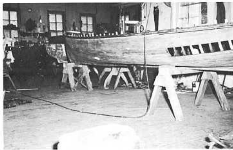
Below: Inside the shop, the paint splattered floor and a 16' row boat needing new pieces
