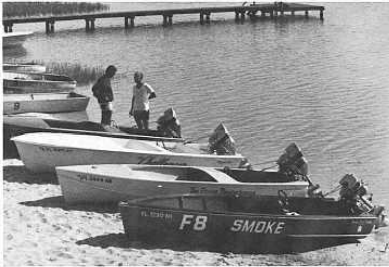
Photo at left: These are the four boats that John took with him on vacation, from front to rear: Barker Todd, 13', with PO-38 Johnson; 1945 Thunderbird, 1st model- fiberglass copy of Barker Todd, Big Four; 1954 Challenger boat, my latest and nicest riding boat, 16' long and fitted with a Big Four P-500 short rod pumper; and 1945 Ramsey with P-500 pumper engine also. My fastest boat, 16', 35 MPH.
