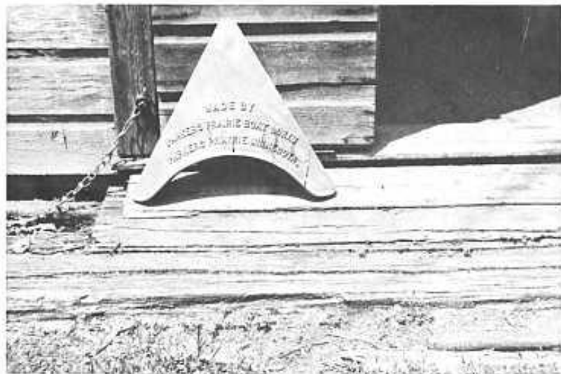
Below: The fancy aluminum breasthook that decorated the bow of most Parker's Prairie boats
