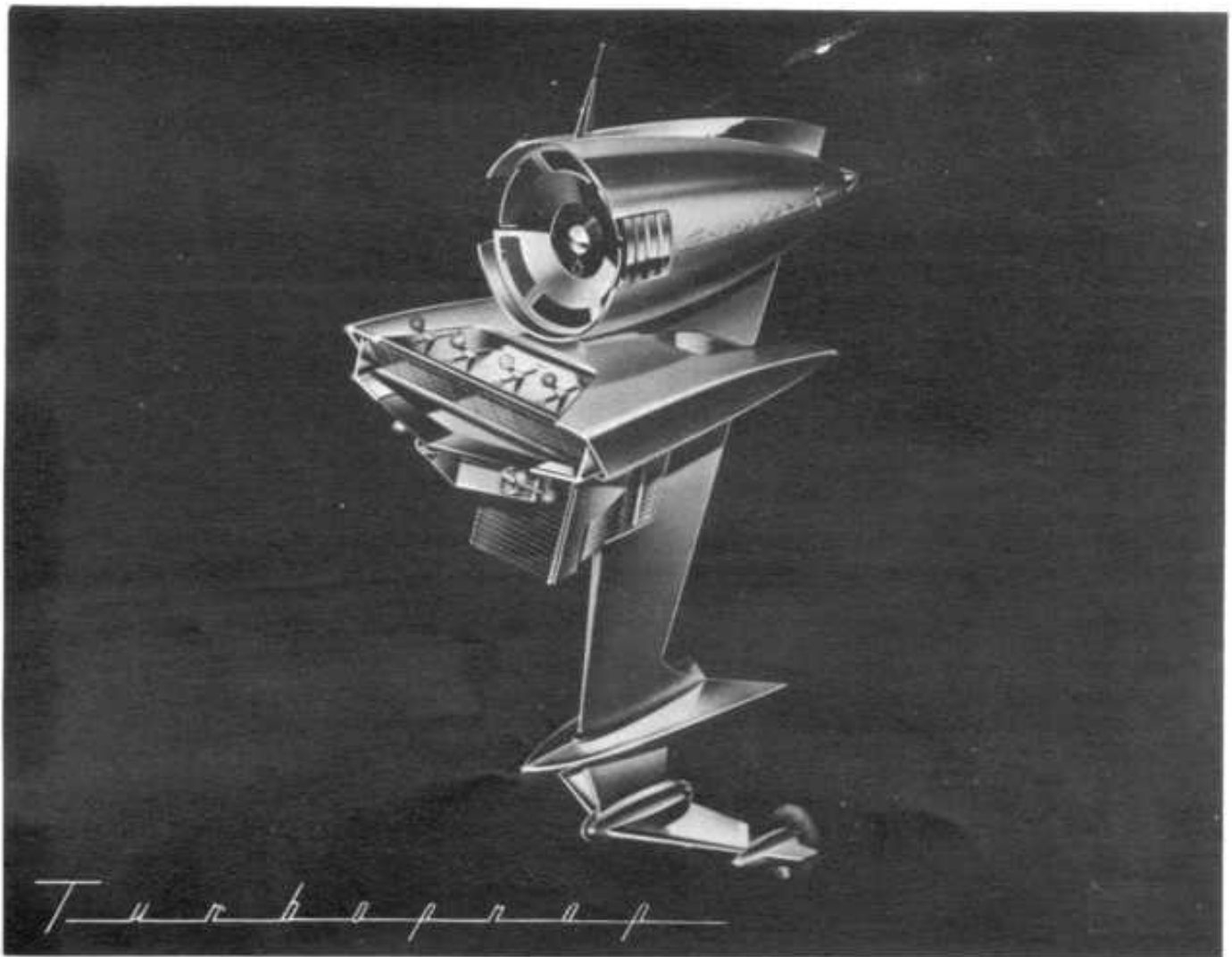
Figure 2. Turboprop. As shown, a gas turbine similar to a jet plane motor drives propellers that allow the boat to be maneuvered like a twin engined cruiser. Air drawn through slots around the speed indicator mixes with gas vapor. The mixture burns rapidly and thrusts against metal vanes which turn the driveshaft. Exhaust gives added push. Other type power sources can be applied to the drive unit. Reverse can be accomplished by mechanical means at present.
