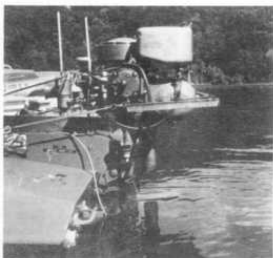
P-50 with P-75 cylinder heads - we experimented. Racing exhaust tube is above water.
