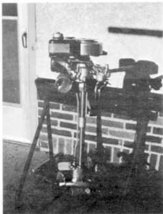
The first Champion, a single, made in 1935. Note the early can type muffler.
