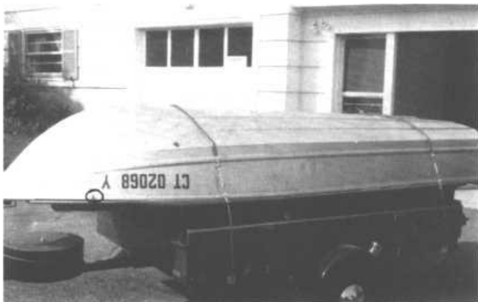
Close up of hold down cables, turn buckles, hose over cable. 4 clamps keep underside cover tight.
