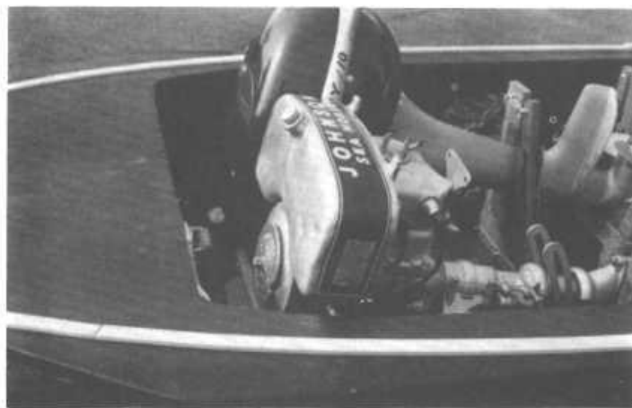
Close up of motor leg clamps. Turn buckles keep leg clamps tight, the motors rigid.
