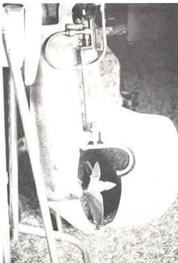
The lower unit showing the curved inlet tube and the pump by-pass leading to the manifold.
