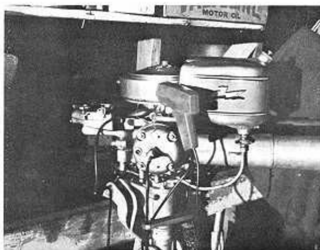
Photo 1. PO Hotrod with timing light and pointer set to determine maximum spark advance.
