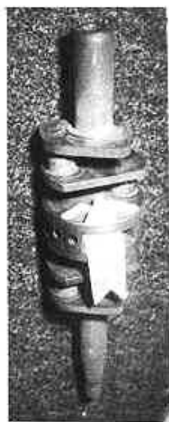
Upper left: Evinrude crankshaft rotary valve from a 16.2 HP Sportfour. Pie-shaped cut is chalked white to show shape.
