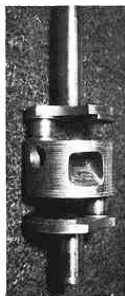
Left: Johnson barrel type rotary valve. This is a KR crankcase. Air/fuel route is more direct than in S-45 type rotary valve.
