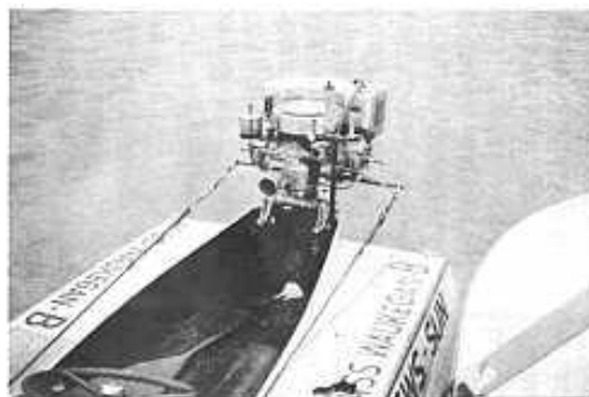
Up and down, two more PR's. Top one has drip type oiler.
