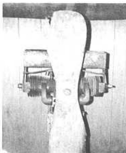
View of the business end. Muffler goes behind prop, between the exhaust manifolds. Note prop width.
