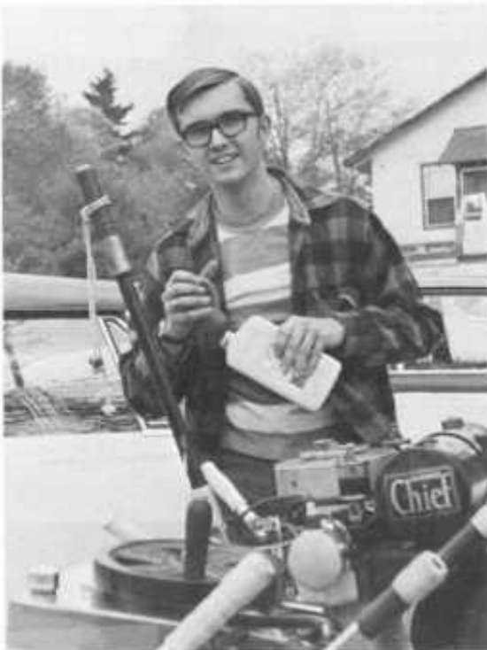
Dick Michel is shown getting his Lockwood Racing Chief ready for action. Dick is putting oil in the Lunkenheimer Oilers.
