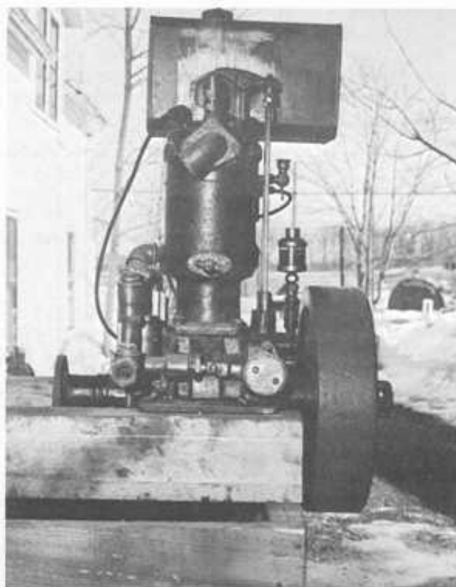
1927 Palmer Model YT-1, single cylinder 2 HP 3" bore X 3-1/2" stroke; 800 RPM. 4-cycle, jump spark. Owned by W. Weidmann
