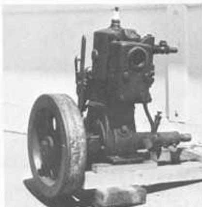
Two views of a 2-1/2 HP Caille Perfection engine, vintage 1908. Note water pump.
