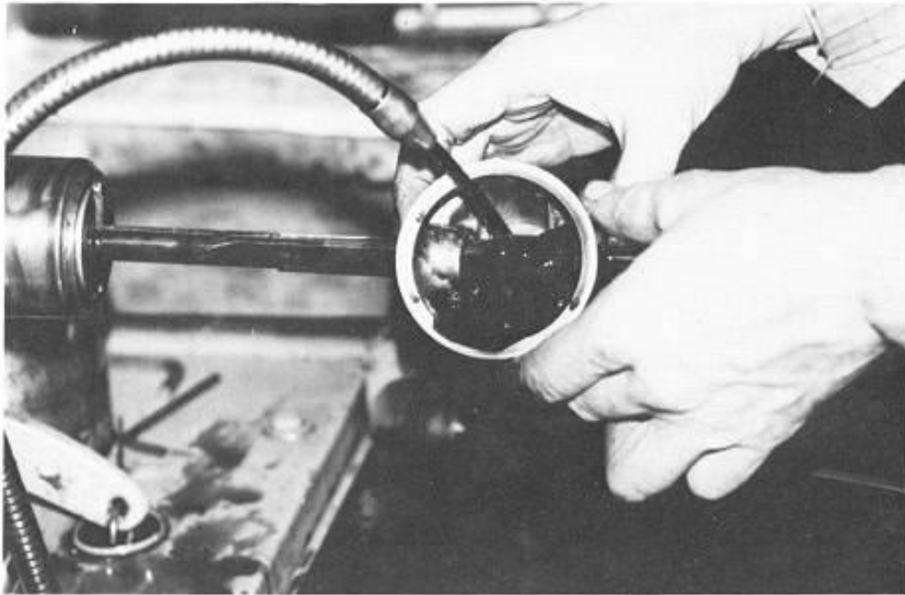
Align honing wrist pin holes for free floating wrist pins.
