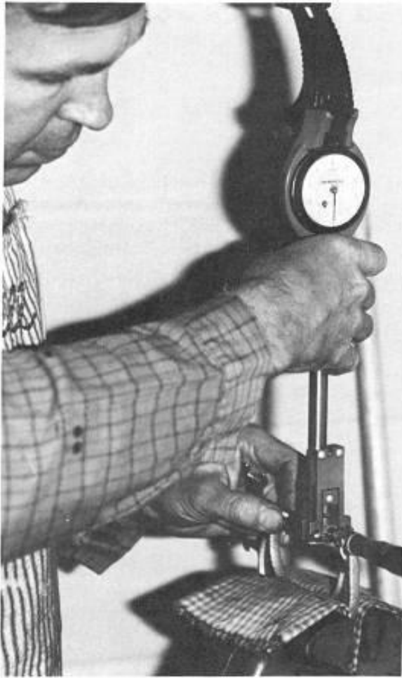
Setting up dial bore indicator for following pictures of Johnson PO cylinder.
