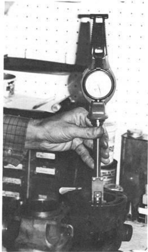
Johnson PO cylinder being measured for roundness and straightness to .0001 inch. Elto Speedster cylinder alongside.
