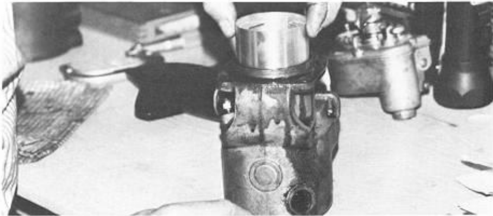
Elto Hi Speed Speedster cylinder being measured by Bill.
