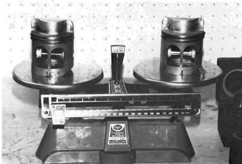
Johnson PR-65 pistons shown on a scale for balancing. Note that attainable accuracy is within one-tenth of a gram. For comparison, a penny weighs 3.3 grams.
