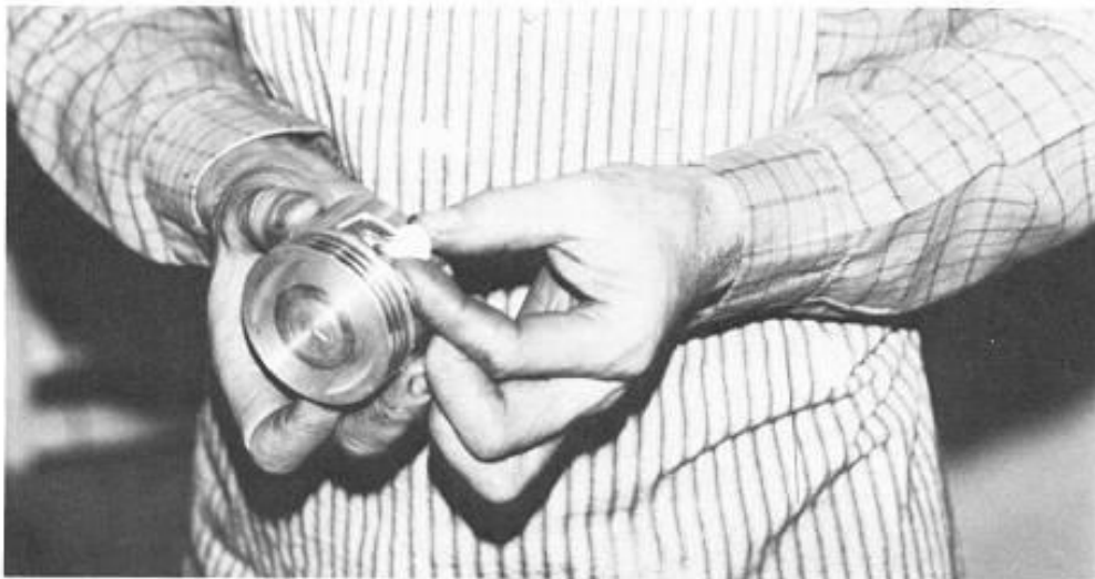
Teflon button stops ruined cylinders caused when antique wrist pin locks break.
