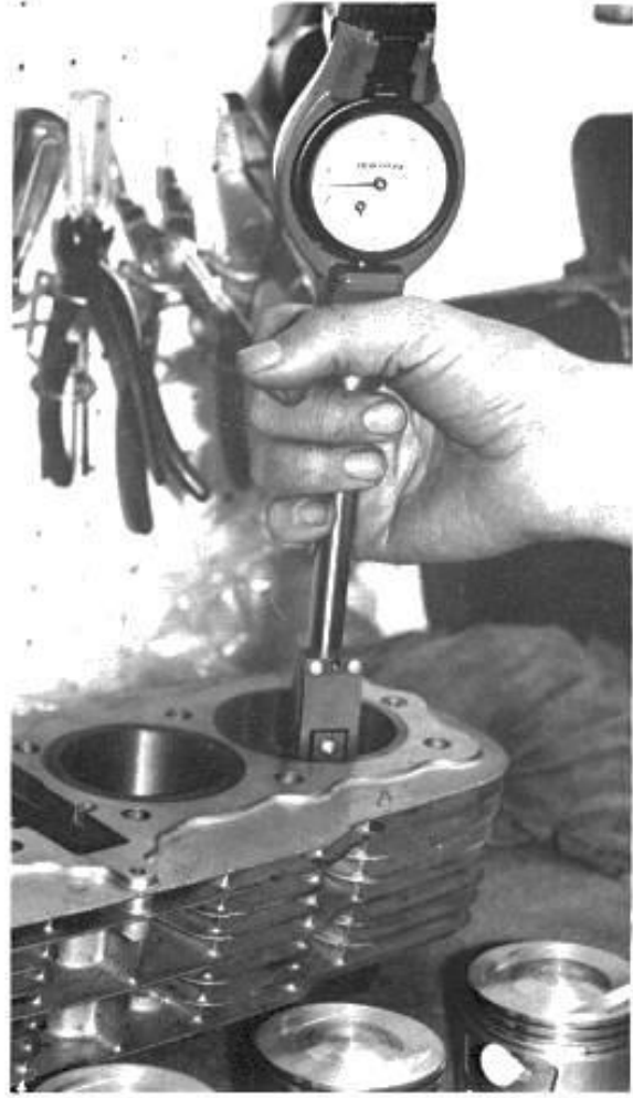
Measuring Honda Four cylinders. Note pistons with Teflon buttons alongside. Is your engine insured against cylinder damage with these?
