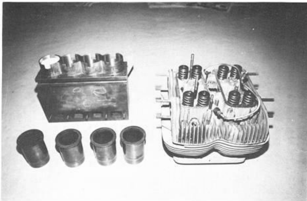
A versatile and competent shop: cylinder head is Ariel Square Four; sleeves are Honda 750; block is a Bugatti.
