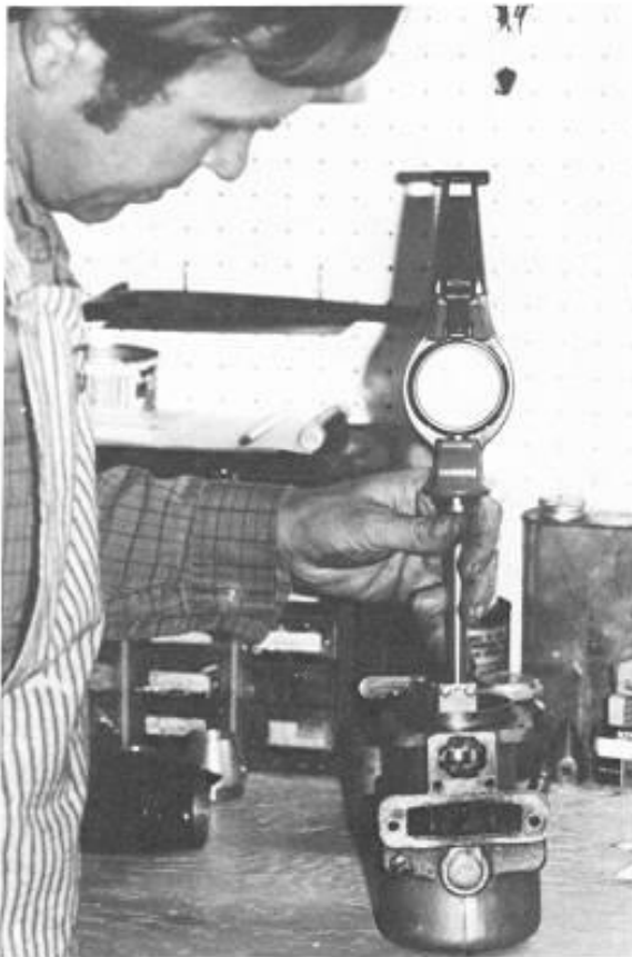
Boring bar working on an Elto Hi Speed Speedster cylinder which, you will note, has a blind [non-removable] cylinder head. Cylinder is at bottom of boring bar.
