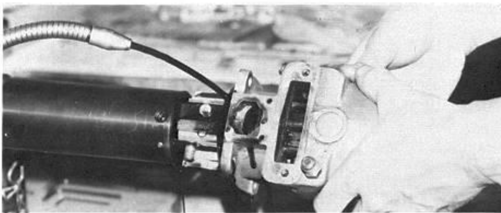
The Elto Hi Speed Speedster cylinder being power honed. This honing process is capable of an extremely high degree of straightness in a blind end cylinder [a non-detachable cylinder head.]
