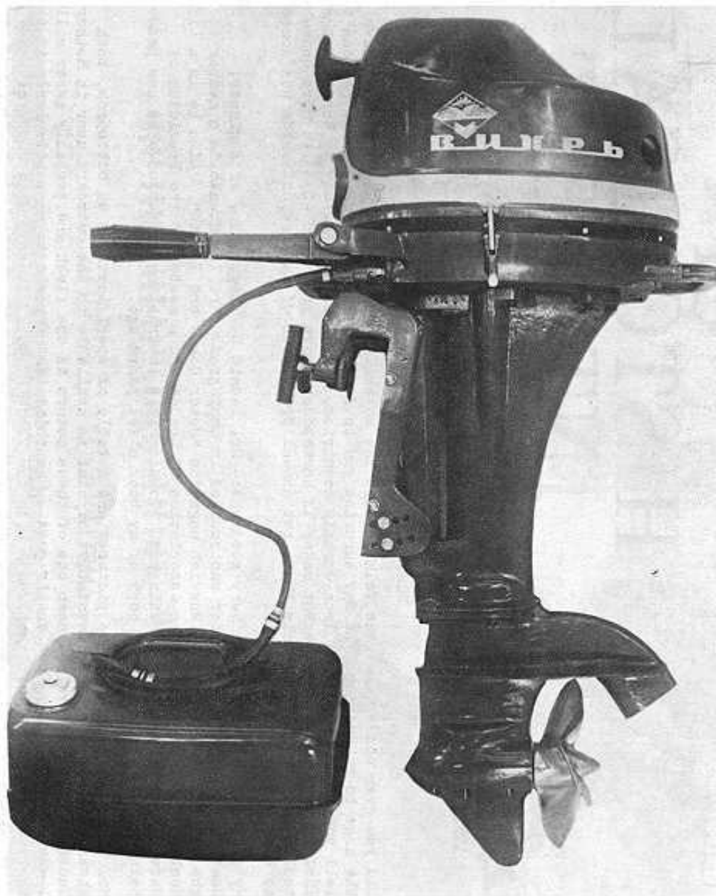
VICHR - 20. (Vertex or Whirl- wind) 20 HP at 4800 rpm. Same motor rated 25 HP at 5000 rpm.
