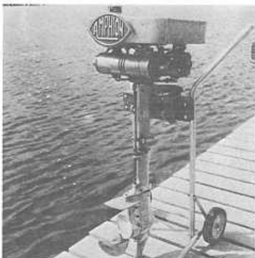
Note the fine tank and lower unit detail. Cyl. heads are air cooled
