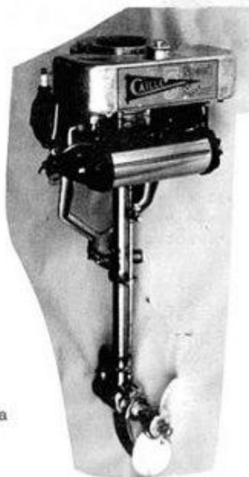
Left- 1917 Caille 2 H.P. Five-Speed Single with rewind starter
