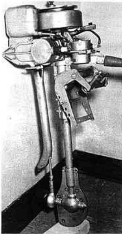
Good view of the lower unit stampings and water pump.
