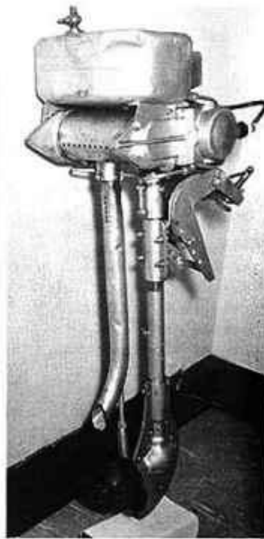
Note stamped pieces of pivot mechanism and transom clamp.
