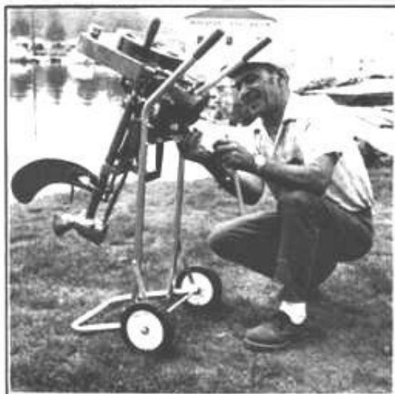
Here's Tony attaching the tiller handle. Photo shows the new gas tank and rudder.
