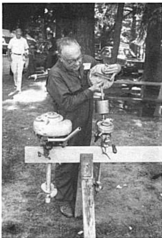
Below left: Mahlon gasses up the show's tiniest antique outboard motor, a \frac{1}{2} horse Elto Pal.
