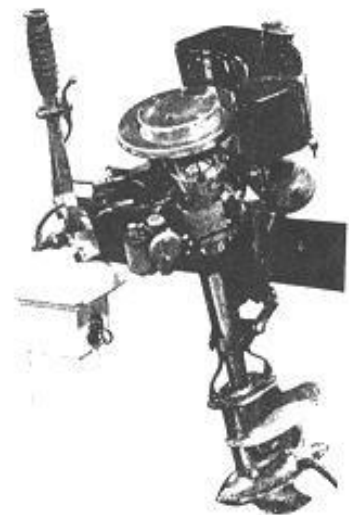
1931 Sharland built by Outboard Motors Ltd., Whitstable, Kent, England. 2-cycle, 4 HP.
