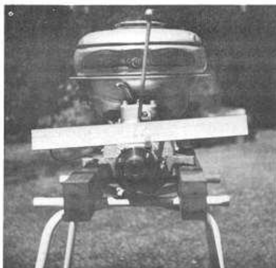
Bendix Eclipse 2 1/2 h. p. single (white line is a ruler, for size comparison.) Front view. Notice reverse gear.
