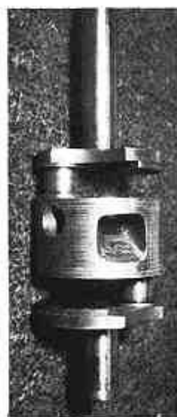
Right: Crankshaft from KR, square port is rotary valve opening for top cylinder. Round hole is blind balancing hole. Port opening for bottom cylinder is 180° from top cylinder port. Barrel is about 1-3/4" thick. Crankshaft is made of 3 pieces, unusual in American engines.
