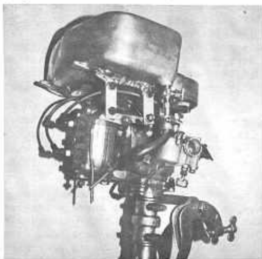
Note raised gas tank, large fuel hose and Tillotson carburetor.
