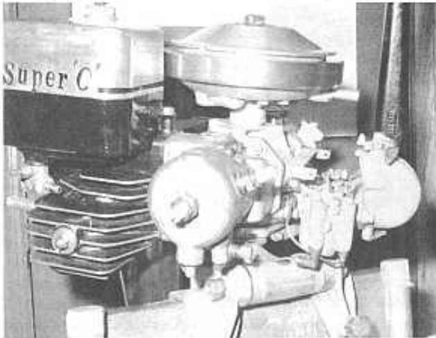
The two optional spark plug locations can be seen here.
