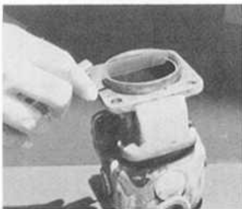
Figure 4 - Measuring ring gap.
