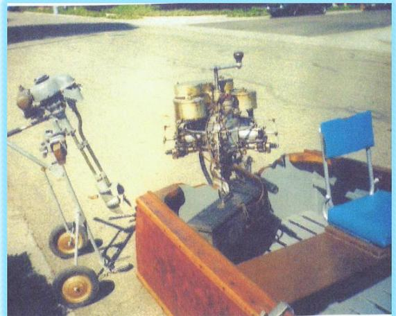
John's grandfather's hand built, five cylinder radial outboard, a very rare motor indeed. Note the oil tank on top of the fuel tank. This motor is of the dry sump design. The small motor is a Power Products Powerhead John's grandfather hand built the lower leg and lower unit. A very gifted man indeed.
