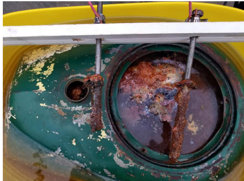
End of hour 4. I will clean the anodes and start again. After three sessions; inside of tank was essentially rust free.
