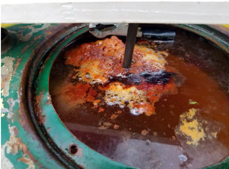
About two hours into the process. Lot of activity! Slowly the rust is being transferred from the metal tank to the steel anode rods,
