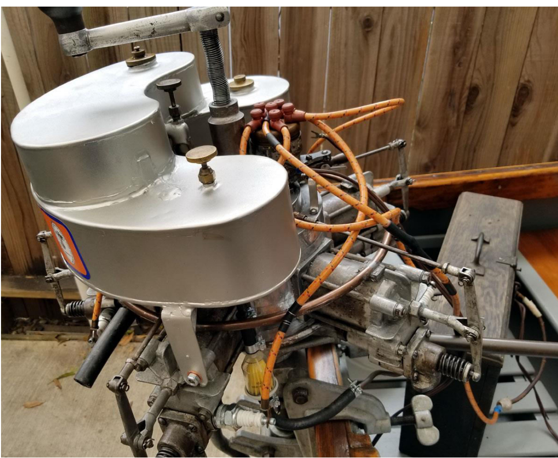
John Van Dykes' 5-Cylinder Radial Outboard Motor. Visible are the two tanks; upper is for oil....lower is for gas. Battery Driven ignition is fed through a distributor. Pushrods for exhaust is visible; the exhaust ports are un-muffled. The Battery Box is visible in the background.
