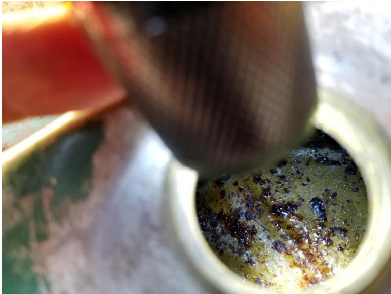
A typical Scott-Atwater Gas Tank from a 1947 7.5HP Outboard. Scott steel tanks are notorious for rust and make a great test for electrolysis rust-removal. The tank is rusty inside and out.
