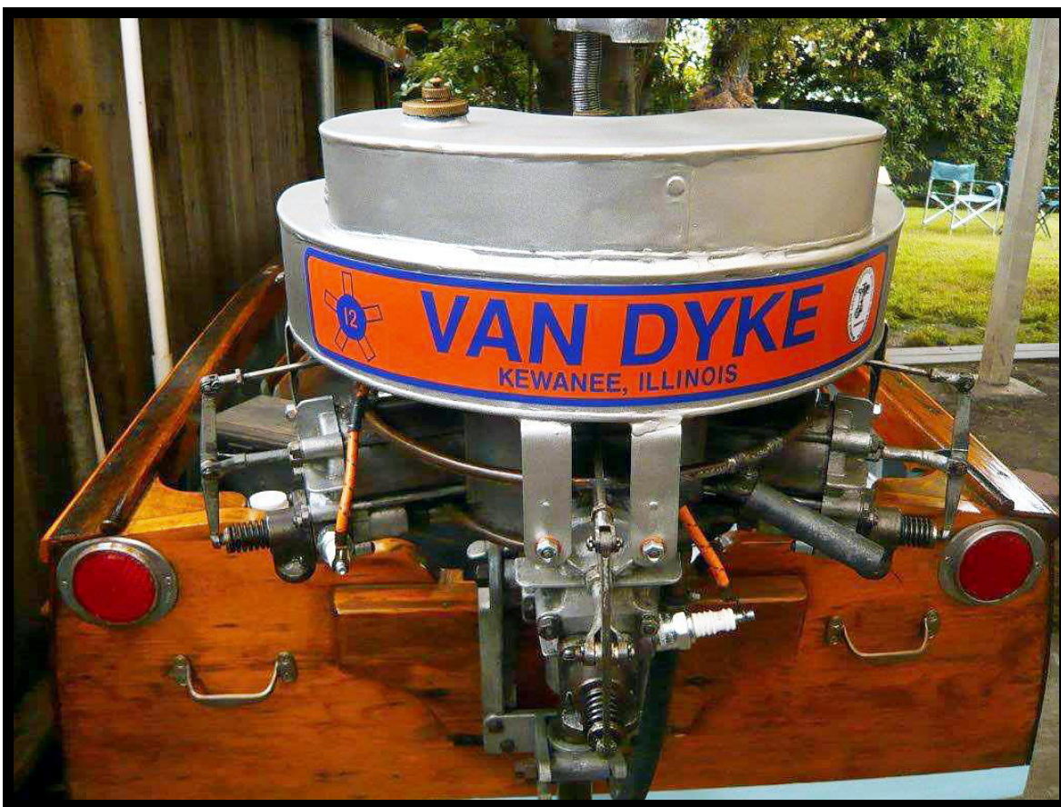
When you make a quality product....why not Put your name on it! Shown is the valve-in valve arrangement; a design patented by John's Grandfather.
