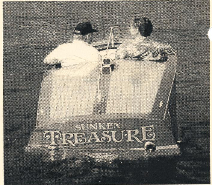
*Accidentally discovered in 1994, in 100 feet of water at the bottom of Lake Tahoe, presumably to have sunk in the 1950's, this 14-foot wooden boat was raised and restored by Wes Selvidge. The biggest surprise was the motor. After 40 years under water, the crankshaft moved when turned with a wrench! When it was broken open, it appeared as if it had just left the machine shop. After a complete rebuild, the engine is both smooth and fast.*
