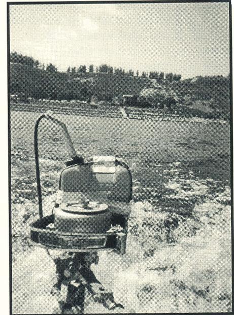
**Tom Lockwood** worked with **George Kent** honing cylinders and reassembling the 1948 Mercury, 3.6 hp KE3 above. They worked so hard that when George brought it to the meet they were really anxious to get it running, so anxious that they duck taped a plastic gas can on it, line and all, and off it went. **Tom Lockwood** says, "If you bring your oars, your motor will always start." "There is truth in that, says George, I did and they ran beautifully."
