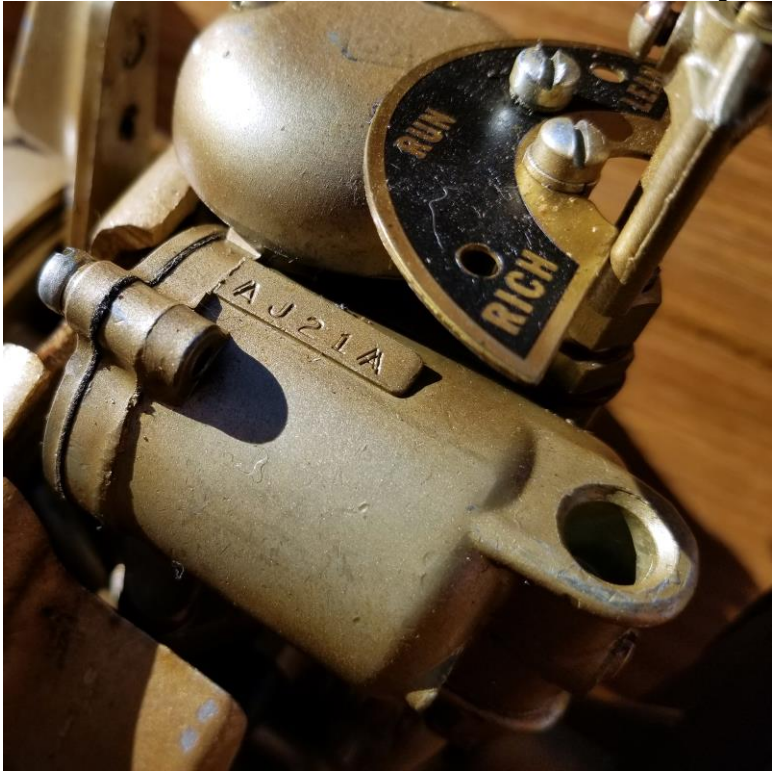
The Tillotson Carburetor on Doug Penn's "Custom-Cratered Neptune"
