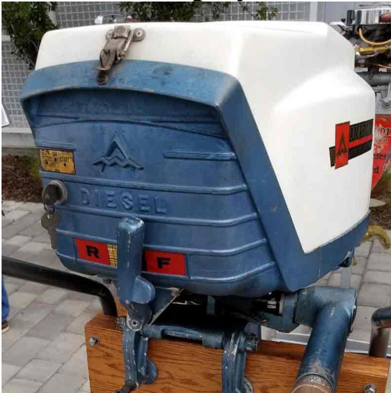
1960-61 AMARC-10 Diesel owned by Tom Lockwood. Manufactured in Inglewood California by American Marc. One Cylinder-Two Pistons 9.8 HP
