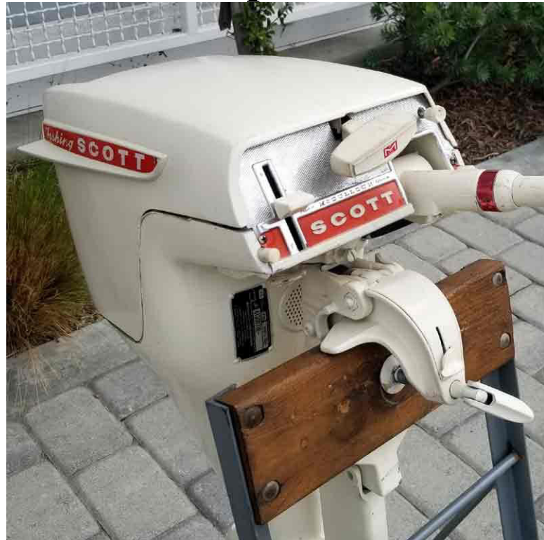
Frank Fowler's near-perfect Fishing Scott. The simplest repair requires removal of the powerhead; right Frank?
