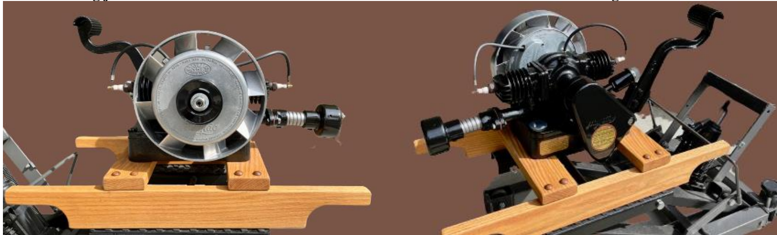
1948 Maytag model 72D-A with Eisemann Magneto 2cyl non-alternate firing 2=cycle engine.
